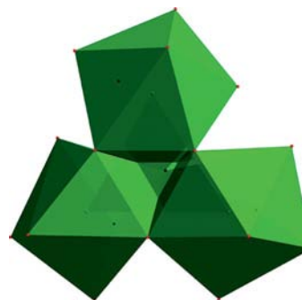
Figure 4. Polyhedral representation of \mu_3\text{-OH} -bridged \text{Gd}_3 triad.
